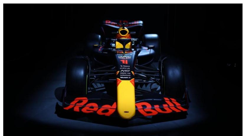
It functions like an inverted airplane wing. The velocity of wind above the wing,  $v_{top}$ , is higher than the velocity of the wind below the wing,  $v_{bottom}$ . This creates a pressure difference due to Bernoulli's equation. This generates downforce, improving the car's grip and cornering performance.
